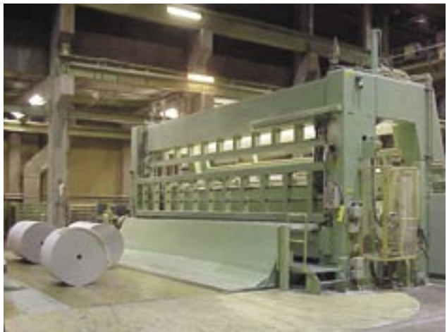
Winder with Rider Roll System RRS
