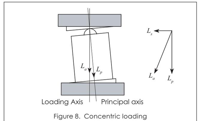
Figure 8. Concentric loading
