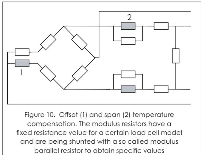
Figure 10. Offset (1) and span (2) temperature compensation. The modulus resistors have a fixed resistance value for a certain load cell model and are being shunted with a so called modulus parallel resistor to obtain specific values
