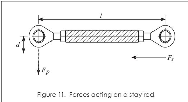
Figure 11. Forces acting on a stay rod
