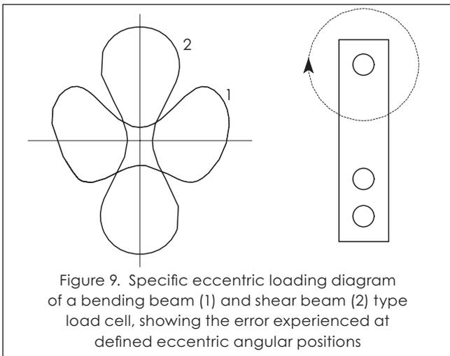
Figure 9. Specific eccentric loading diagram of a bending beam (1) and shear beam (2) type load cell, showing the error experienced at defined eccentric angular positions
