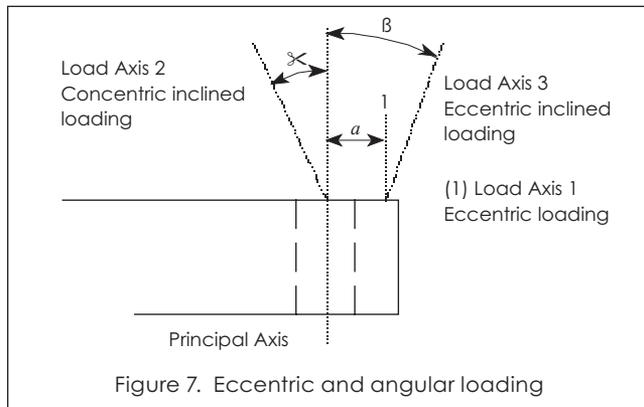
Figure 7. Eccentric and angular loading
