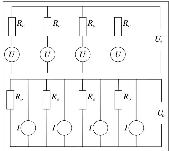
cell is now represented as a current source, driving current through the parallel combination of the load cell source impedances, where  $I = U / R_o$ .
