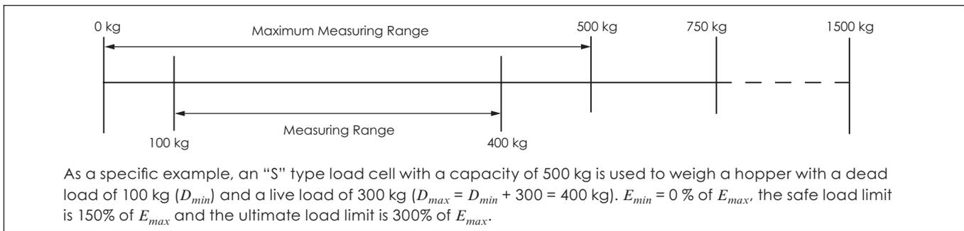
As a specific example, an "S" type load cell with a capacity of 500 kg is used to weigh a hopper with a dead load of 100 kg ( $D_{min}$ ) and a live load of 300 kg ( $D_{max} = D_{min} + 300 = 400$  kg).  $E_{min} = 0\%$  of  $E_{max}$ , the safe load limit is 150% of  $E_{max}$  and the ultimate load limit is 300% of  $E_{max}$ .
