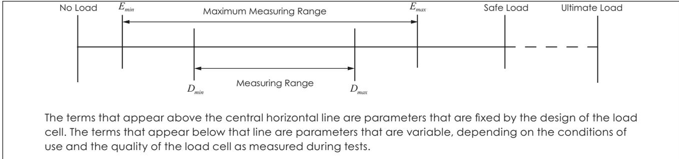
The terms that appear above the central horizontal line are parameters that are fixed by the design of the load cell. The terms that appear below that line are parameters that are variable, depending on the conditions of use and the quality of the load cell as measured during tests.
