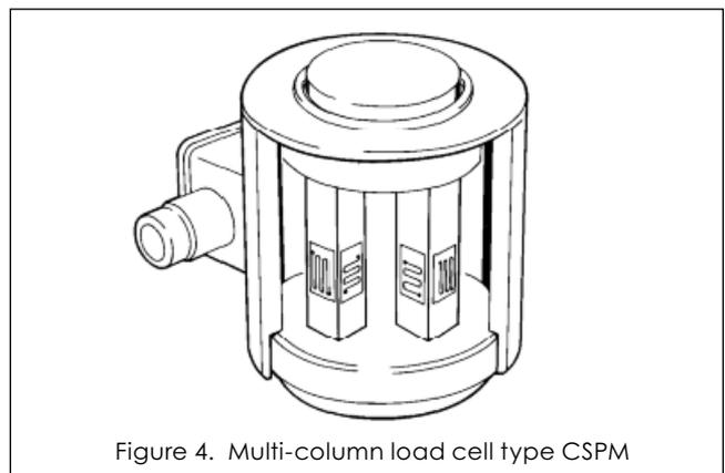
Figure 4. Multi-column load cell type CSPM
