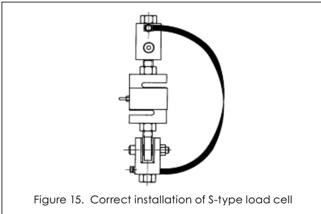
Figure 15. Correct installation of S-type load cell
