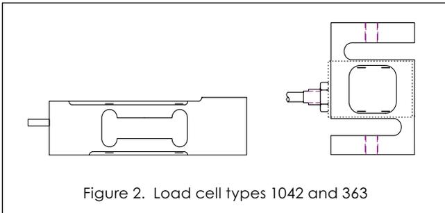
Figure 2. Load cell types 1042 and 363
