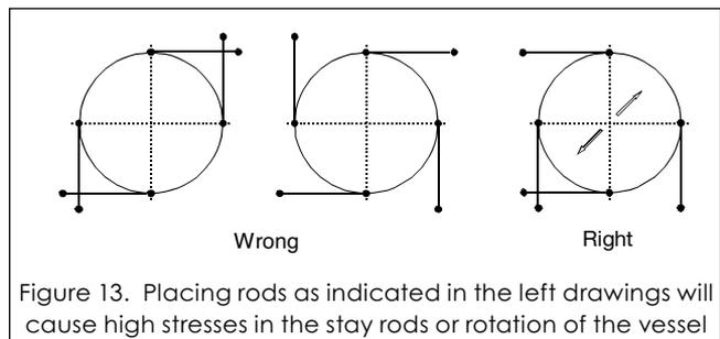
Figure 13. Placing rods as indicated in the left drawings will cause high stresses in the stay rods or rotation of the vessel
