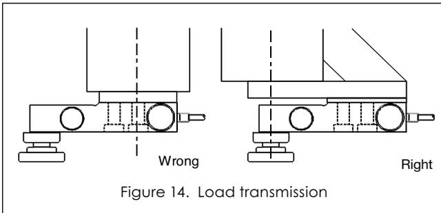
Figure 14. Load transmission
