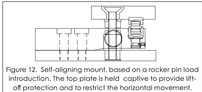
Figure 12. Self-aligning mount, based on a rocker pin load introduction. The top plate is held captive to provide lift-off protection and to restrict the horizontal movement.
