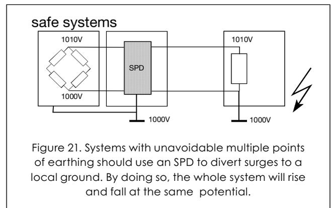
Any device which works by diverting large currents to a local ground must have a low impedance connection to that ground. This means that the bonding connection must be of low resistance (well below  $0.5 \Omega$ ), short in length and as direct as possible without sharp bends. Verify the earth connections at least twice a year and coat all connections with a good antioxidant grease.
