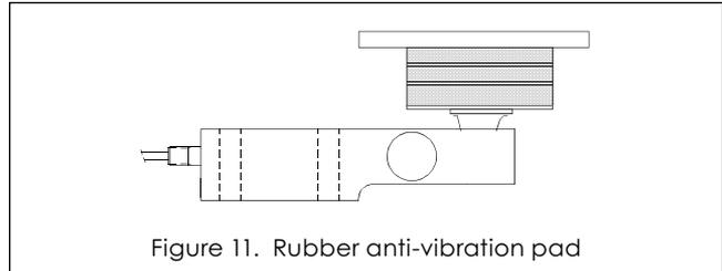
Figure 11. Rubber anti-vibration pad
