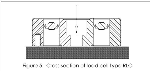
Figure 5. Cross section of load cell type RLC
