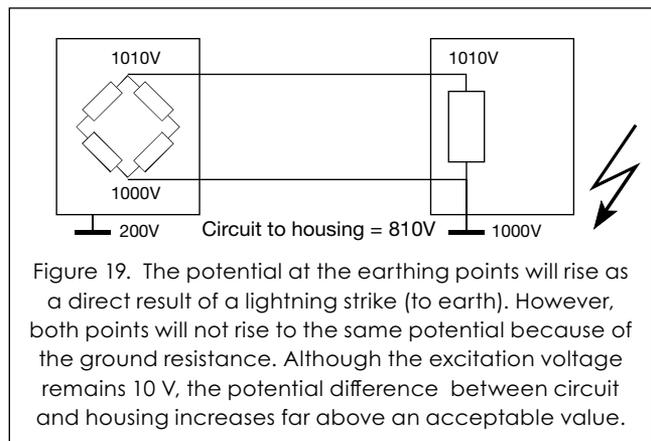
It should be recognized that a high potential difference between housing and load cell circuit can be caused by:
