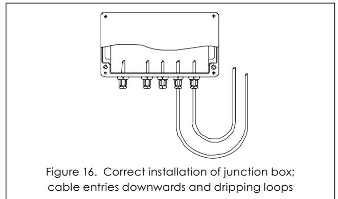
Figure 16. Correct installation of junction box; cable entries downwards and dripping loops
