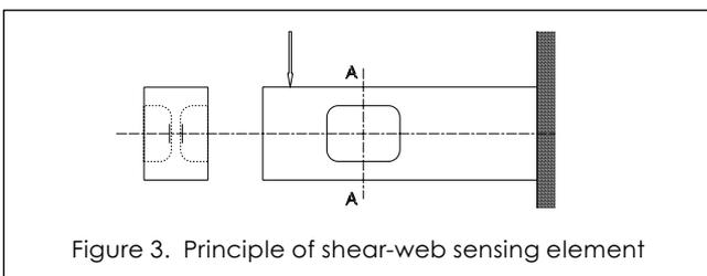
Figure 3. Principle of shear-web sensing element
